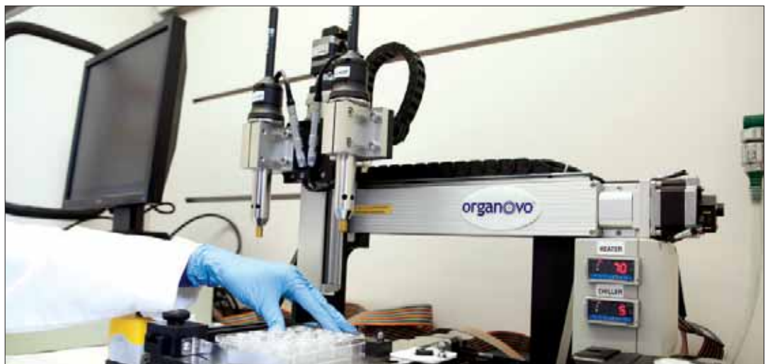
Real human cells can be assembled by a machine into a three-dimensional tissue. By layering various types of skin tissue, Organovo can better mimic the complexity of actual human skin. Melissa Jacobs
