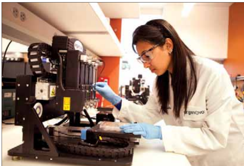
Melissa Jacobs Vaidehi Joshi, a senior research associate at Organovo, uses human cells as "ink" to build organ tissue with the company's 3-D printer, the NovoGen.
